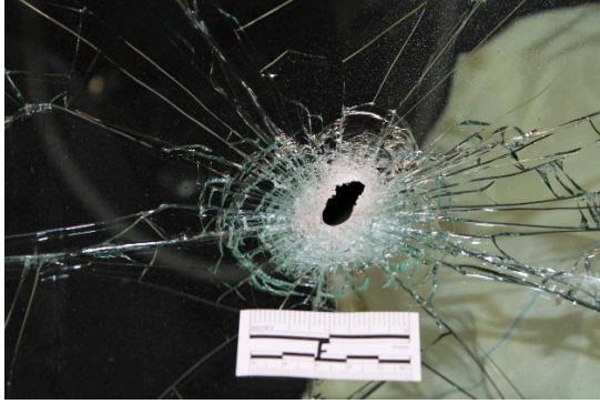
Sticker G: Small defect in glass of front windshield located in front of the steering wheel of the vehicle. The defect appears to have glass shards pushing outside to the exterior of the car instead of inside to the interior of the car.
