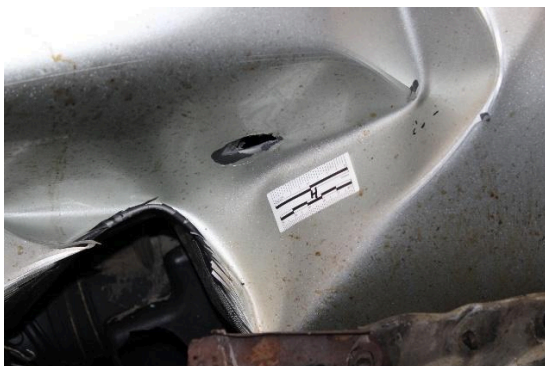
Sticker H: Defect located on the right side of the vehicle's hood near the driver's side front fender. There is chipped paint and the defect is oblong with a wider base to the left and a smaller base to the right. The defect appears to perforate into the interior of the hood.
